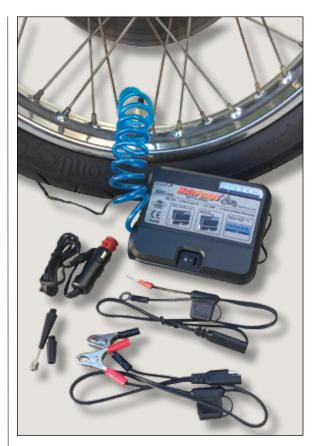
the pump draws 4.75 amps (and be sure to change the fuse back to the smaller one if your charger or other device calls for it).
